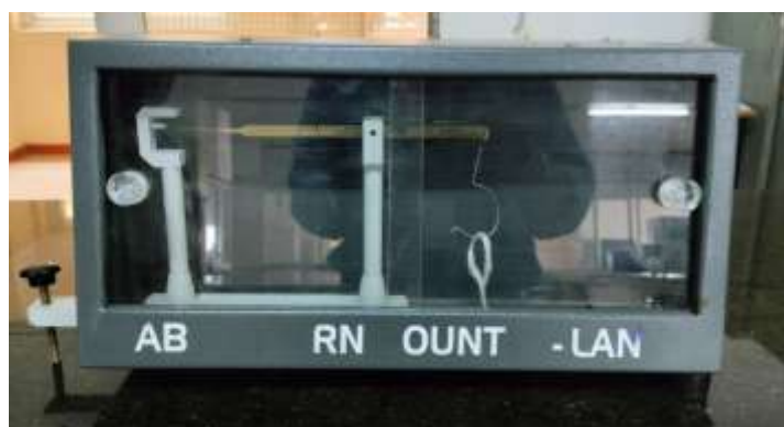
PLATE 3: BEESLEY BALANCE YARN COUNT TEST
