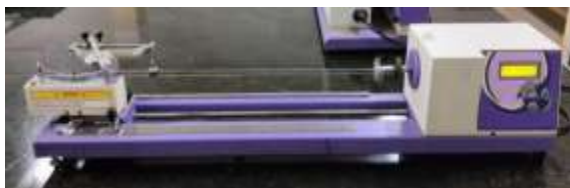
PLATE 4: YARN TWIST TESTER
