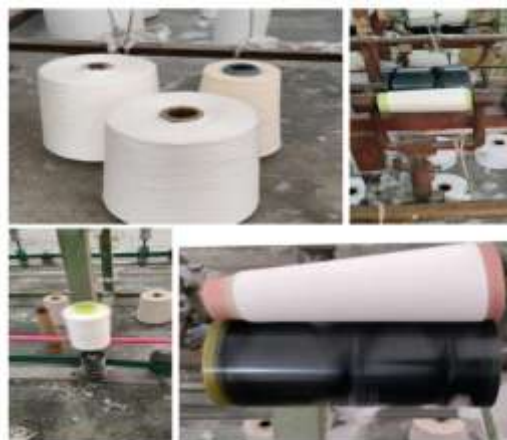
PLATE 1: TWISTING PROCESS OF SINGLE PLY 100% CHP YARN
